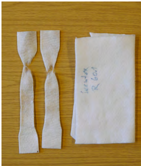
Figure 1. Test sample of geosynthetics (Naue Secutex R601). Left: Virgin sample (surface weight 600 g/m 2 . Right: after artificial ageing in autoclave (80° C, p(O 2 ) = 30 bar, 21 days) and checking on tensile testing machine (Zwick).
