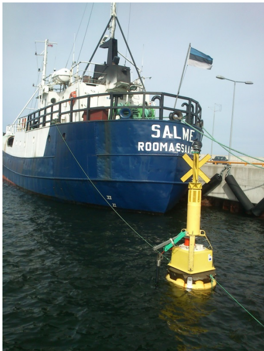
Figure 1. Water column profiler testing on the background of R/V Salme. Photo by Fred Buschmann.
