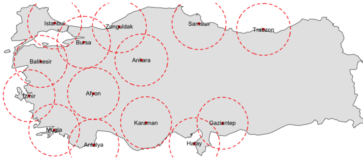
Figure 2. The distribution of 14 radar network over Turkey. Precipitation products of six radars (Istanbul, Bursa, Balikesir, Izmir, Mugla, and Afyon), which were taken from TSMS were evaluated manually to describe the characteristics of the precipitation types.
