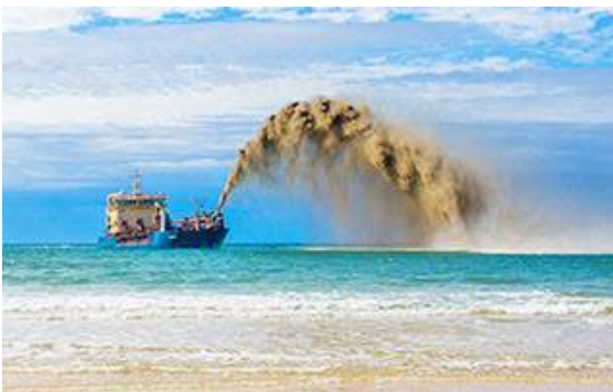
Figure 3. The dredge 'Balder R' rainbowing sand into the nearshore. (Source: Gold Coast City Council)
