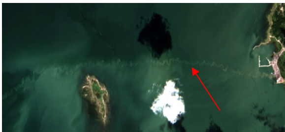
Figure 4. Suspended sediment mixed into the water column by Heltermaa-Rohuküla ferry imaged by Sentinel 2 (10 m spatial resolution)
